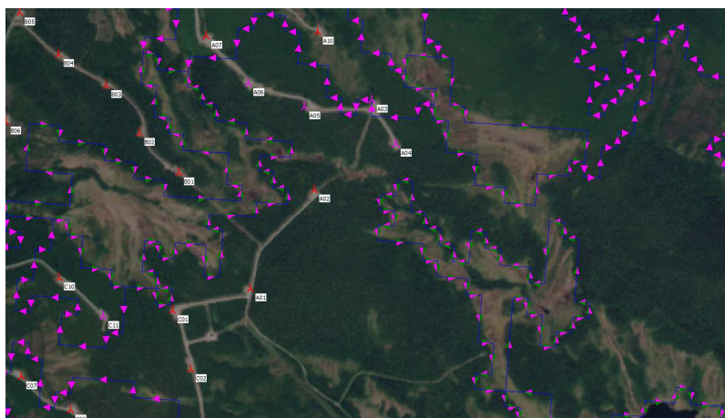
Figure 1: Left: CORINE data in windPRO. Right: Roughness lines from CORINE 2012 on top of Sentinel 2 imagery (site in Sweden).
